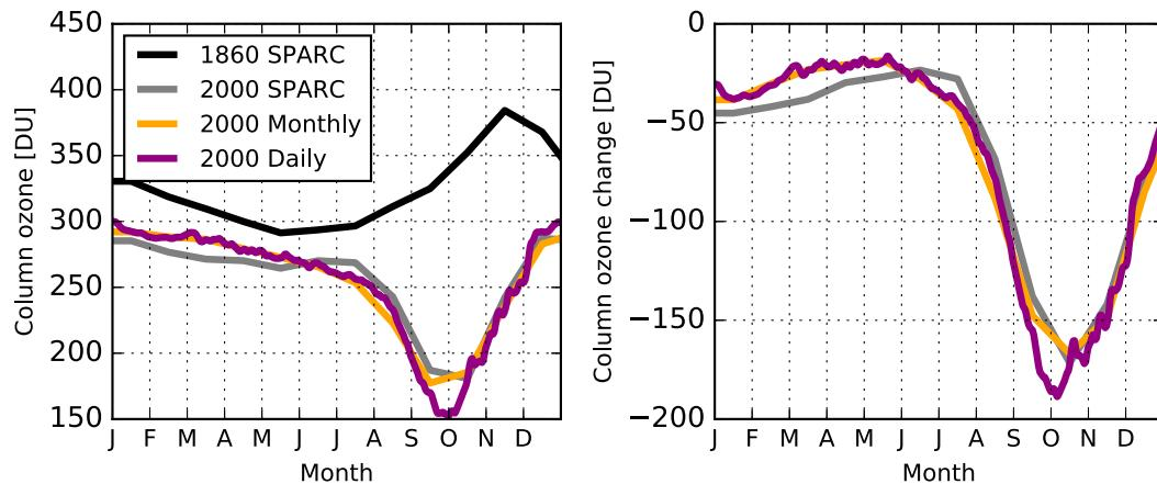
FIG. 1. (left) Seasonal cycle of polar cap ( $70^{\circ}$ – $90^{\circ}$ S) averaged column ozone in the control simulation (1860 SPARC) and the perturbation simulations with year-2000 ozone prescribed with monthly and daily mean values from WACCM-SD. (right) Difference of 2000 ozone and 1860 ozone simulations. Also shown for comparison is 2000 column ozone from the SPARC dataset and the difference between 2000 and 1860 SPARC values (gray line).
